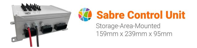
The **Sabre Control Unit** fits in the back of any storage cabinet or can be installed in the boot compartment. The control unit houses 16 control circuits, 16 channel override switches (for emergency operation), status lights, GPS receiver, satellite modem (if fitted), circuit breaker and reset button, tank monitor system and CAN-Bus and CI-BUS systems.
